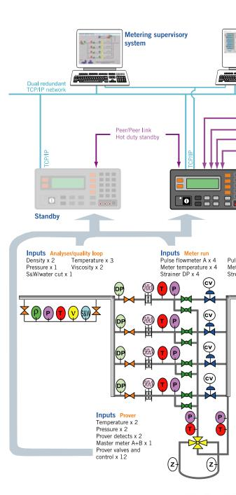
The schematic above shows a typical 4 meter run metering station. Here one flow computer could be used for all instrumentation including the prover. For critical applications the redundancy offered by hot duty/ standby is often preferred.
