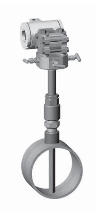
KB Series system with integral 3-valve manifold and direct mounted 4301 DP transmitter
